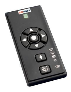
CANbus Control System is based upon **NMEA 2000**, a combined electrical and data specification for a marine data network for communication between marine electronic devices. It is defined and controlled by the US based National Marine Electronics Association (NMEA). NMEA 2000 connects devices using Controller Area Network (CanBus) technology originally developed for the automotive industry.
